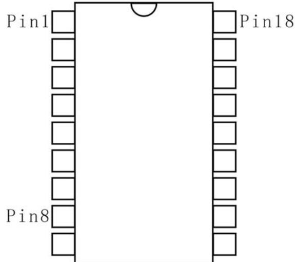
Just in case there aren't any labels printed on the PCB board, you still can easily figure out the "L" and "H" states yourself: After power is hooked up to the system, use a Voltmeter to measure the contacts on both sides of the column of eight pins. Voltage level on each side should be consistence. If one side is "H", the other side should be "L". "H" level voltage can be measured only when signal is transmitting/receiving.
